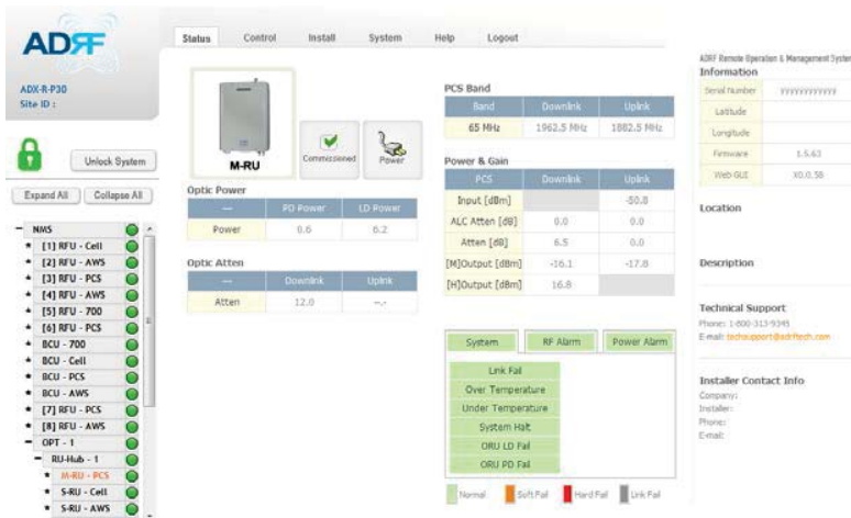
Figure 8-28 Status – Remote Module
