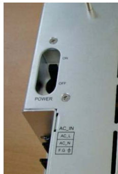
Figure 3-31 HRU AC Switch
