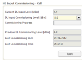
Figure 8-70 RFU Commissioning (Install – RFU)
