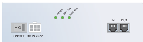
Figure 3-31 Ports at the rear panel (Slave RU)
