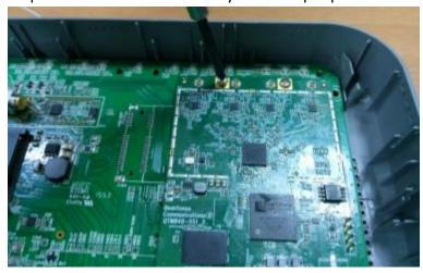
Step4: Assemble the antenna, 2pcs per unit
