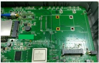
Step2: Assemble XW866G in the miniPCle socket.
