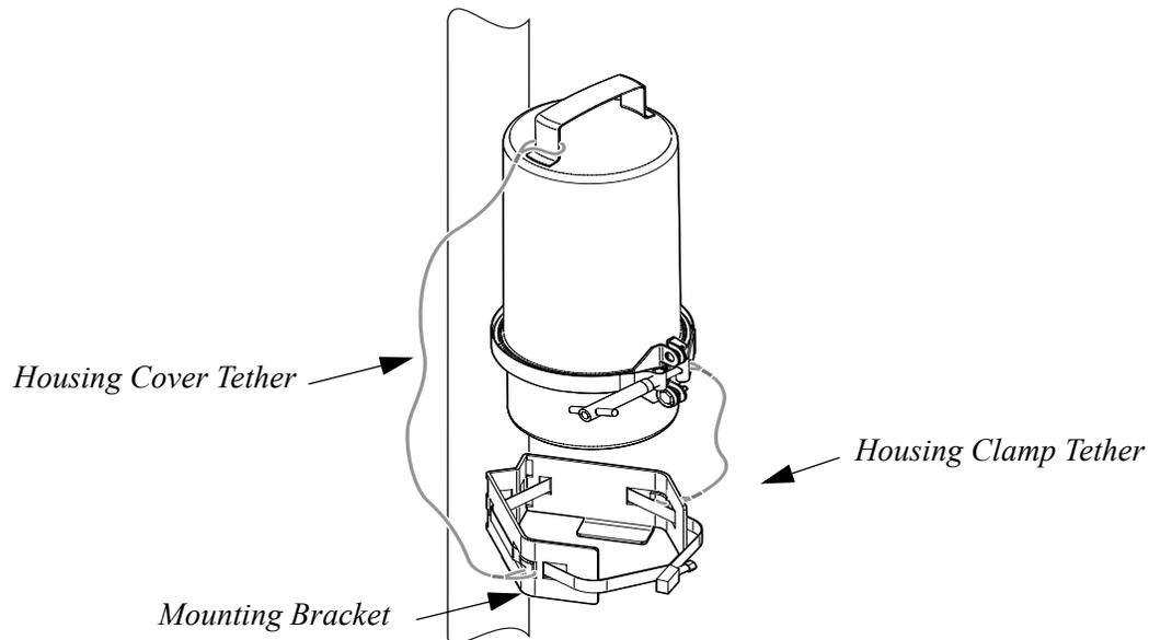
**Figure 3. Connecting the TRACER 3202 Rope Tethers**
