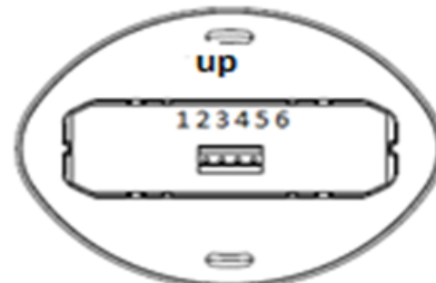
External reader backside view / terminal block pin ordering details
