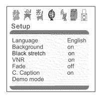
Fade: The FADE control allows for the picture tube to warm up and gently turn on, which can help prolong the life of the picture tube.
