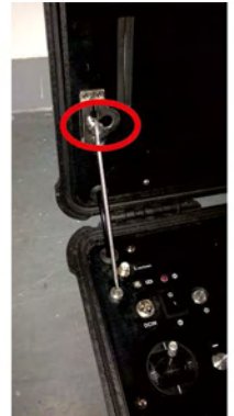
Slip the support rod leftward to fix it
