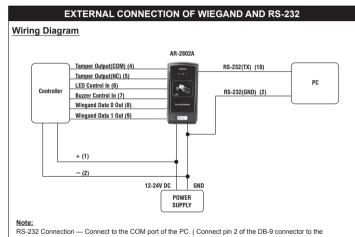
terminal (10); connect the terminal (2) GND of the device to pin 5 of the DB-9 connector.)
