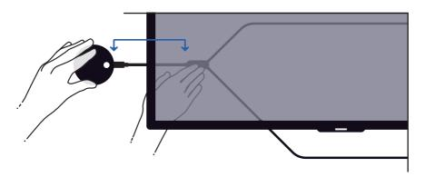
**Keep the Aircord straight** and stick the cable splitter to a surface behind the TV.
