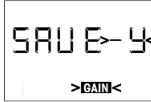
If you want to save the new setting, push the jog switch briefly. The display will show your new gain setting in dB and the "GAIN" label will be flashing.
