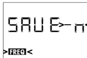
Push the jog switch briefly. The transmitter will stay tuned to the original frequency and the display will revert to the following screen:
