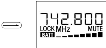
**Frequency Screen:** Carrier frequency in MHz, battery capacity bars. The "MUTE" label appears if the microphone is muted.
