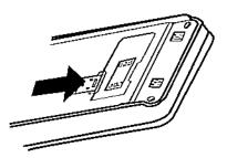
5. Place the battery on the back of the phone and slide it up the body of the phone until it locks into place.
