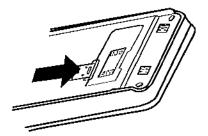
3. Insert the RUIM card ensuring that the bevelled corner is on the bottom right and the golden contact area is facing downwards.
