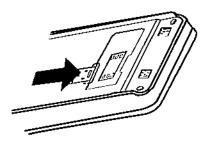
5. Place the battery on the back of the phone and slide it up the body of the phone until it locks into place.
