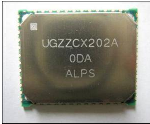
Fig 1. Top View of Bluetooth Transmitter “UGZZC-2###”
