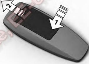
1. Remove the cover. To do so, press the cover, arrow 1, and push forwards, arrow 2.
