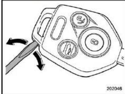
1. Open the key head using a flat-head screwdriver.
