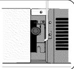
Position valve water line as illustrated and secure with small plastic clip located in ice maker kit.
