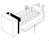
When frozen, the cubes are moved up and out of the mold.
