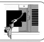
3 Tuck bottom portion of valve inside machine compartment and fasten valve to cabinet with 1/4" screw from step 1.
