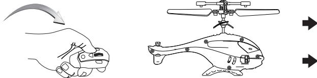
Tilt the controller forward and the helicopter will move forward.
