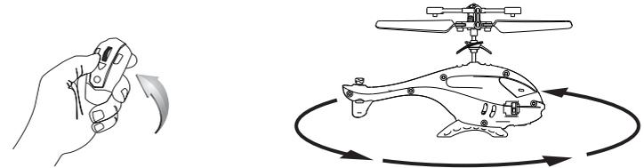
Tilt the controller left and the helicopter will spin counterclockwise.
