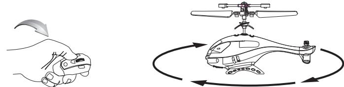
Tilt the controller right and the helicopter will spin clockwise.
