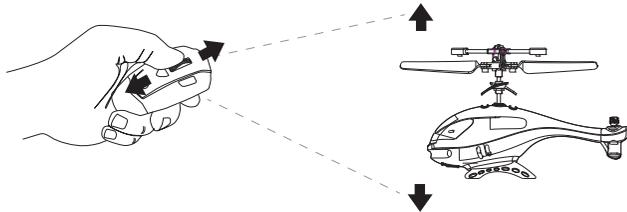
Roll the Throttle wheel forward to increase the speed of the main rotor, and roll the Throttle wheel backwards to decrease the speed of the main rotor. The helicopter will rise or descend accordingly.
