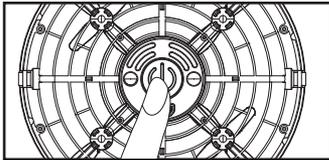
7. When done playing make sure to turn the power off by depressing the power button for 3 seconds (see power button diagram on pg. 3 ) All the lights will turn off.
