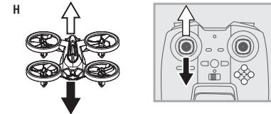
While in the air, move the left Throttle stick left and the AIR RACER™ 2.0 will rotate left.
