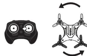
Move the Throttle stick left and the X20 will rotate left.
