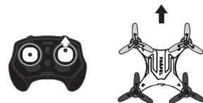
Move the Direction Control up and the X20 will move forward.
