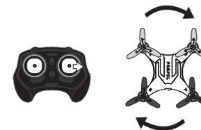
Move the Throttle stick right and the X20 will rotate right.
