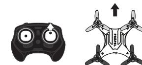
Move the Direction Control up and the X20 will move forward.
