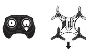
Move the Direction Control down and the X20 will move backward.
