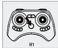
**Tips:** You also can move the two control sticks simultaneously down inside or outside corners, hold them till the blades start spinning. Release the control sticks and push the throttle stick slowly to take off manually (see diagram H2).
