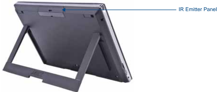
FIG. 20 IR transmitter window on the MVP-9000i-GB
