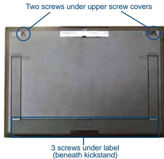
FIG. 114 Placement of screws on the back of the MVP-9000i
