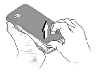
b. Remove the battery if inserted
