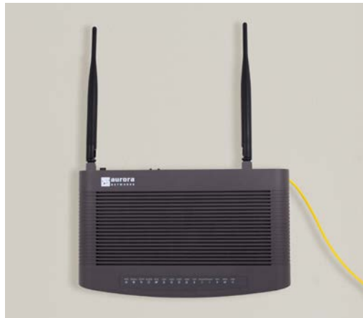
Figure 10 EPON Multi-service Gateway Wall-mounted
