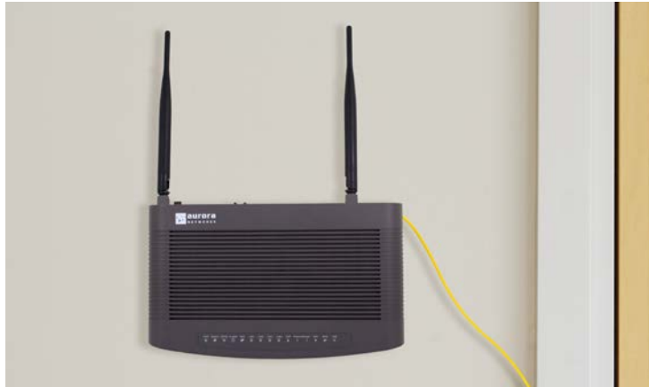
Figure 8 EPON Multi-service Gateway Wall-mounted onto Fiber Tray
