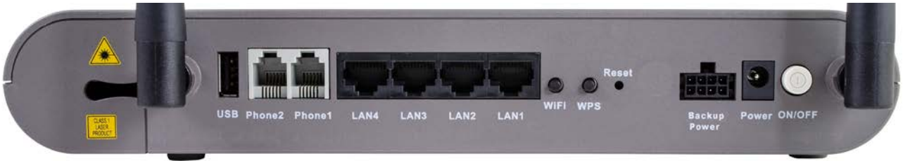
Figure 2 Rear Panel Ports on the ONT-2-E4020iWn
