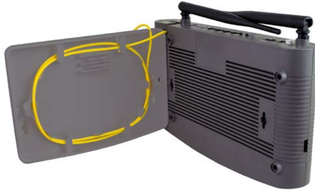
Figure 12 Snapping the ONT onto the Fiber Tray
