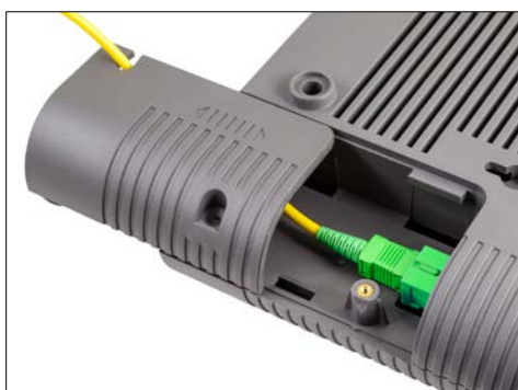
Figure 3 SC/APC Optical Fiber Plugged into Optical Network Interface
