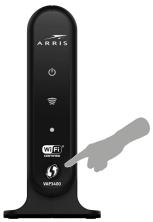
4. The Client's Wireless Link LED lights: You have now established a secure wireless connection between the Access Point and the Client. Check to ensure the Wireless Link LED lights, indicating the VAP is functioning as a Client. You now can begin streaming video content to your set-top box or boxes.
