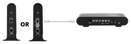
Connect the power adapter to the VAP, plug the adapter into a wall outlet and set the Power switch to the ON position. You'll see the power LED on the unit's front panel light green, indicating the unit is powered.
