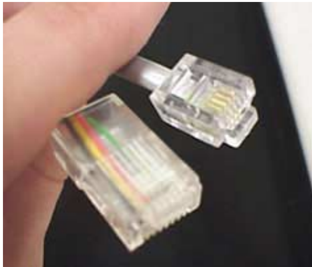
The plug on the left is RJ-45; the plug on the right is RJ-11 – use only RJ-45.
