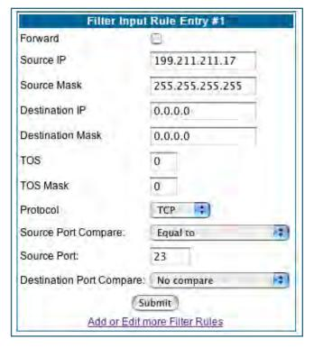
The type of higher-layer Internet protocol the packet is carrying, such as TCP or UDP
