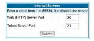
**Web (HTTP) Server Port:** To reassign the port number used to access the Motorola Netopia® embedded Web server, change this value to a value greater than 1024. When you next access the embedded Motorola Netopia® Web server, append the IP address with port number>, (e.g. Point your browser to <a href="http://210.219.41.20:8080">http://210.219.41.20:8080</a>).
