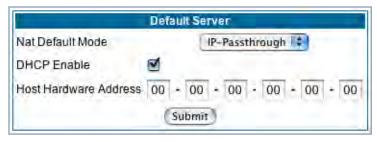
The **Host Hardware Address** field displays. Here you enter the MAC address of the designated IP-Passthrough computer.
