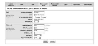
Figure 4-13 Wireless LAN Configuration
