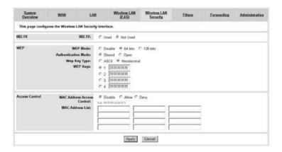
Figure 4-14 Wireless LAN Security Configuration
