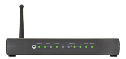
The RSGu3500 has four ports and wireless capabilities. You can connect up to four devices to your RSGu3500.
