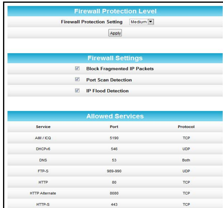
Figure 28 – Firewall Protection Level Screen
