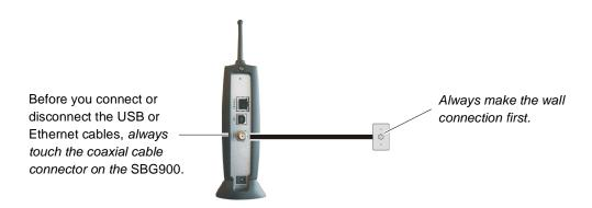
To avoid potential shock, always unplug the power cord from the wall outlet or other power source before disconnecting it from the SBG900 rear panel.
