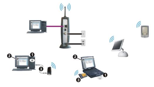
To set up the SBG900, on a computer wired to the SBG900 over Ethernet or USB, perform the procedures in "Setting Up the Wireless LAN". Do not attempt to configure the SBG900 over a wireless connection.
