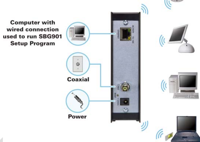
Figure 5 Sample Wireless Network Connections
