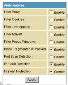
Checkmark **Enable** for each Web filter you want to set for the firewall, and then click **Apply**. The Web filters will activate without having to reboot the SBG941 Configuration Manager.
