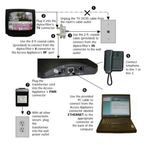
**Note**: To ensure proper operation and UL compliance of product in the USA, use only the approved power supply included.
