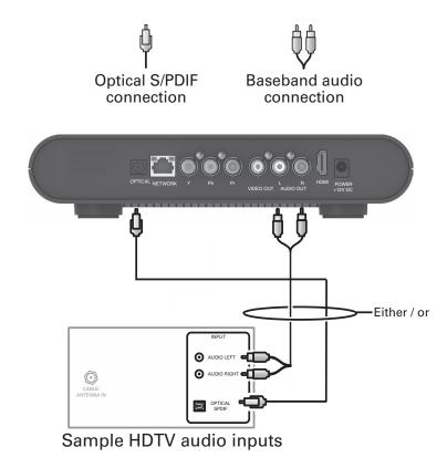
If your equipment supports it, use the OPTICAL S/PDIF output. Otherwise, use the AUDIO OUT L and R connectors. In most cases, S/PDIF offers better audio quality, including support for Dolby Digital 5.1 Surround Sound.
