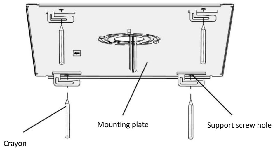
3、 Remove the mounting plate, drill holes in the marked position with electric drill, and install the wall anchor into the hole;
