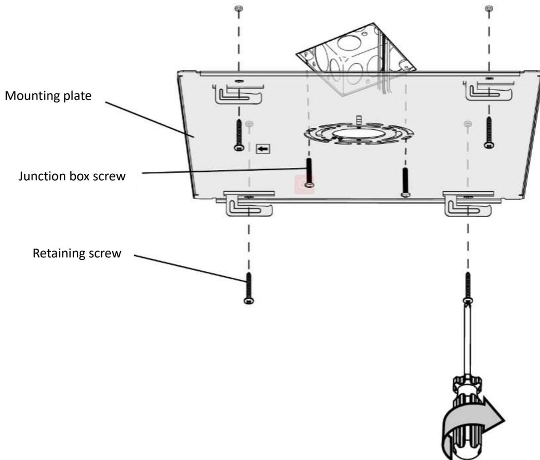
5、 As shown in the figure, hang the hook on the mounting plate and connect the wires as required;
