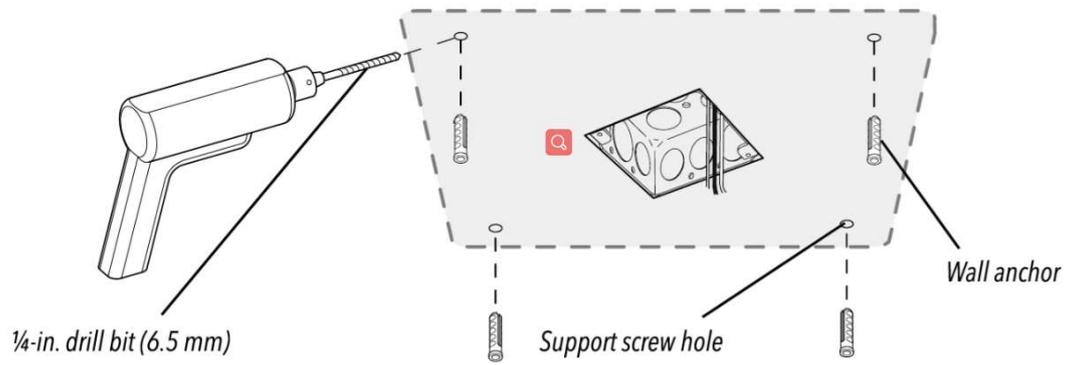
4、 As shown below, install the mounting plate;
