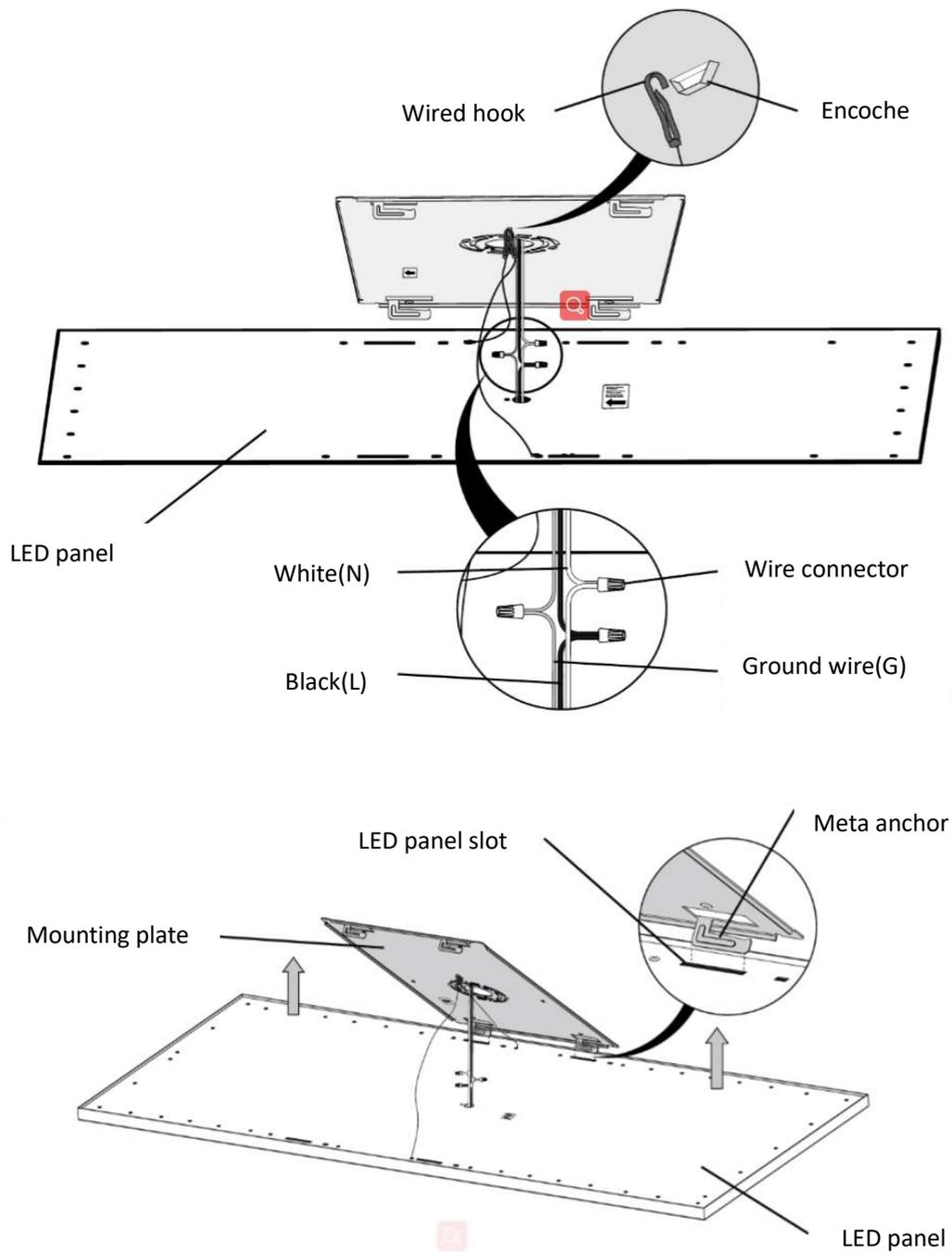
6、 Assemble the panel light onto the mounting plate as shown;
