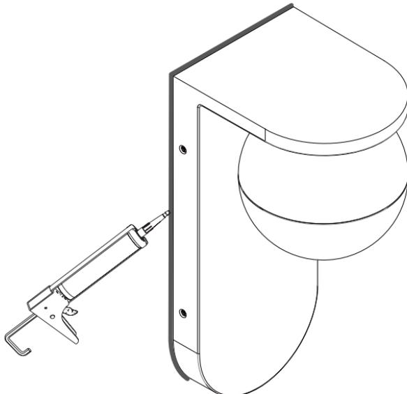
**NOTE:** We recommend keeping the bottom unsealed. To maintain a drainage area in case of water infiltration.
