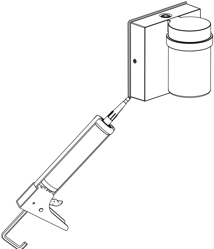
**NOTE:** We recommend keeping the bottom unsealed. To maintain a drainage area in case of water infiltration.
