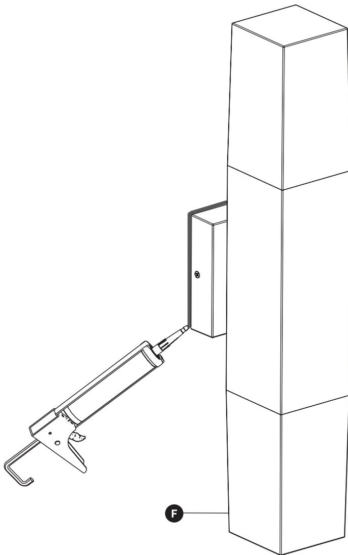
**NOTE:** We recommend keeping the bottom unsealed. To maintain a drainage area in case of water infiltration.
