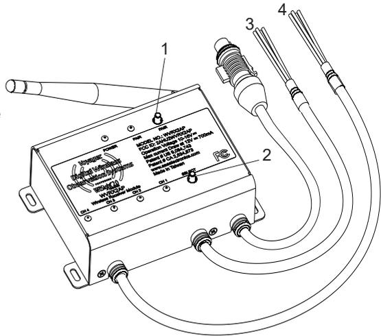
Make sure transmitter module is unpowered at first. Within 50 seconds of activating the pairing process on the receiver module, apply power to the transmitter module, and upon successful pairing, the receiver module and monitor screen will display "PAIRING SUCCESSFUL" message for 1~2 seconds with the status LED steady ON and display Camera image.
