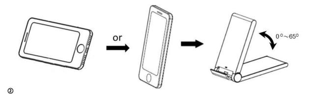
2, Put your mobile phone vertically or horizontally on the wireless charging stand and ensure its center aligns with the center of wireless charger. Besides, you can adjust your wireless charging stand angle from 0 to 65 degree you want while using.
