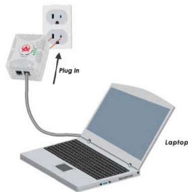
Figure 1-2: Example of How Your PlugLAN 8660 SmartBridge AV Ethernet Adapter Fits into Your Network
