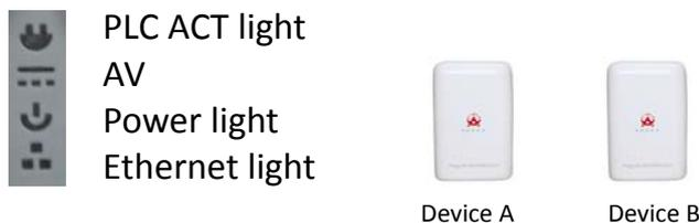
1. Select a PlugLink 500 MIMO ETH (Device A) and plug into an AC outlet. The POWER light indicator should be lit solid green.
