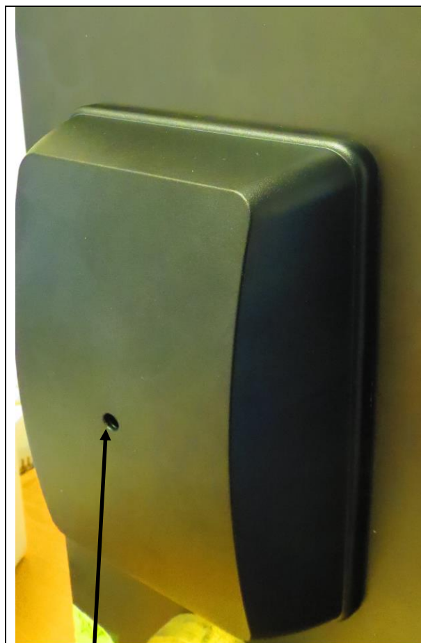
Open with Torx T20s screwdriver
