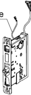
Figure 19: The lock case is the only part which is specific for ANSI (DA).
