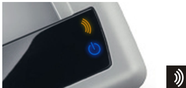
Figure 7-7: position and design of RFID activity indicator LED
