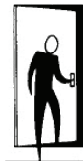
Left Hand: Hinges on left, opens inward. For handed locks, specify LH .
