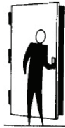
Left Hand Reverse: Hinges on left, opens outward. For handed locks, specify LHR .
