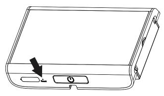
Using a small tool, press the reset button for 5 seconds to reset the door viewer to factory defaults.
