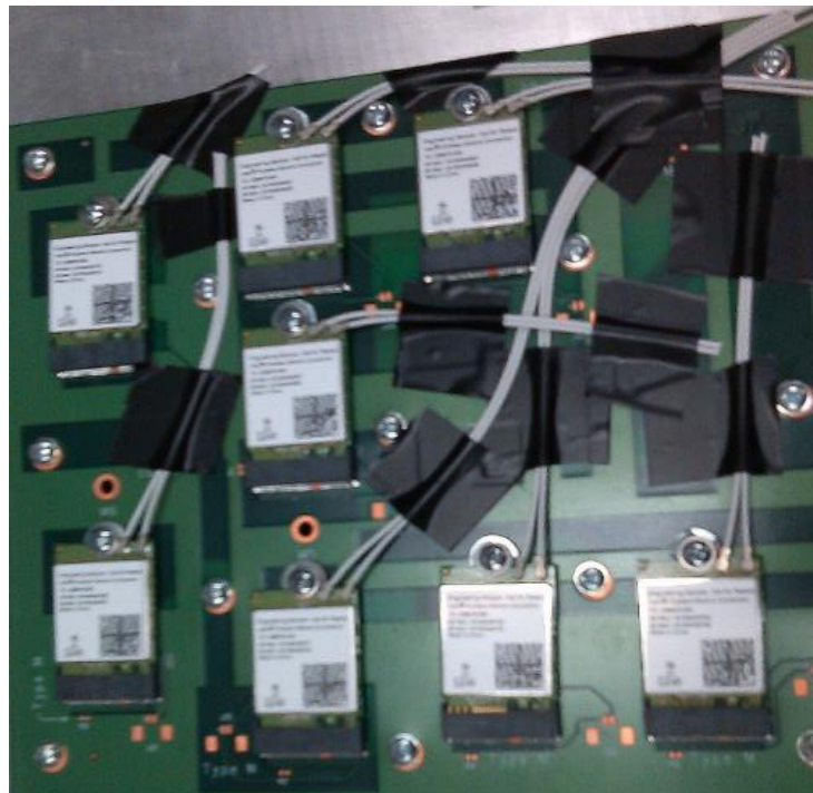
Figure 9-2 M.2 cable retention
